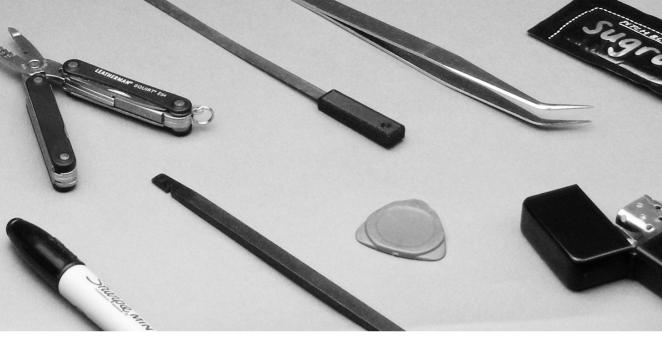
**Leatherman Squirt ES4**. Tiny multitool that can cut/strip wires, has files, knife, and pliers. Killer addition to any toolkit.
