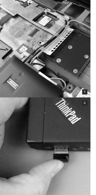
internal antennas inside the X200, and the SIM card slot (underneath the battery), to give you 3G and GPS connectivity. If you really wanted to go all out, you could create a custom adapter that adds a hardware switch, so you control when it's turned on and off.
